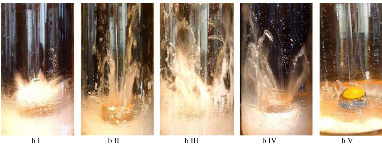
Figure 4 – Splash after impact of metal jet with the bottom of teeming ladle of various design
