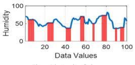
Figure 16 – Stuck at fault
