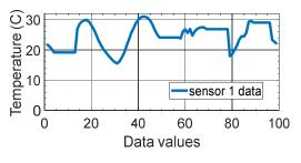
Figure 3 – Stuck at fault
