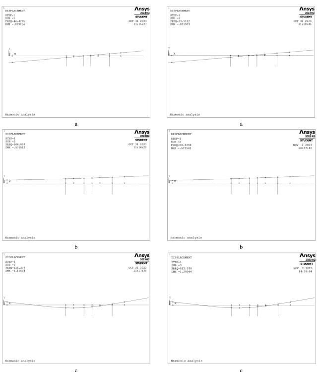
Figure 8 - 1st (a), 2nd (b), and 3rd (c) forms of self-oscillations of the pump rotor at nominal clearances
