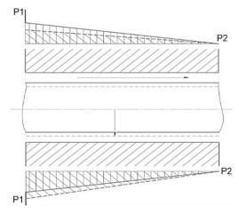
Figure 3 – Pressure distribution in slotted seals
