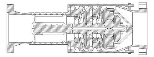
Figure 1 – The developed pump ECW 8-63-150
