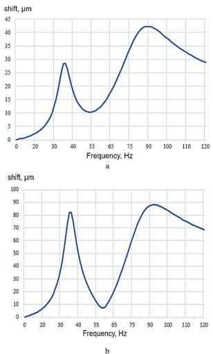
Figure 7 - Amplitude-frequency characteristics at the points of excitation of the front seal of the first-stage impeller (a) and the radial gap of the hydroheel (b) at doubled clearances
