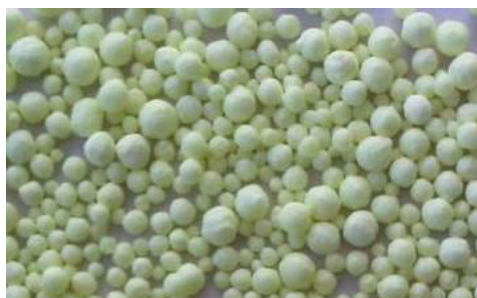
Figure 6 – Photo of the gaseous sulfur granules (3–6 mm)
