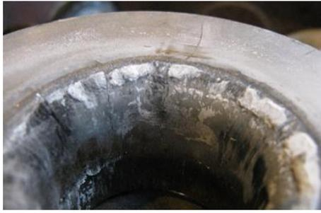
Figure 1 – The wear of the matrix for the pipe press [5]
